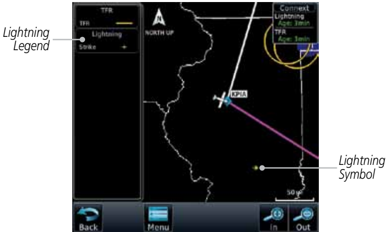
Figure 12-79 ConnexT Data Link Lightning and Legend
