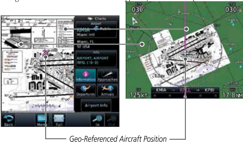
Figure 7-22 Areas of Chart Info Removed For Map Overlay and Geo-Reference
