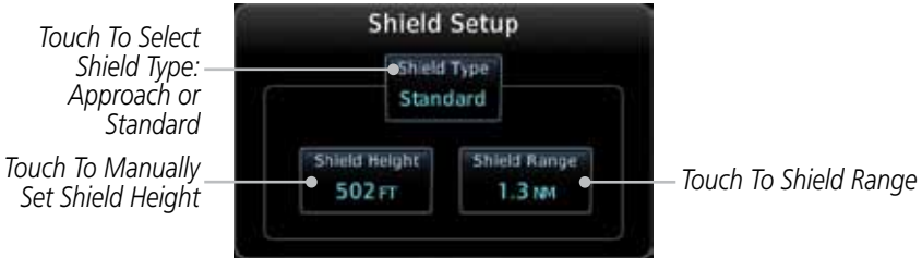
Figure 10-29 TCAD 9900B Shield Setup for En Route, Standard, and Terminal
