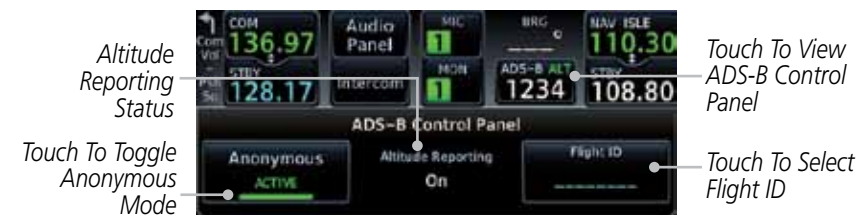
Figure 2-10 ADS-B Control Panel
