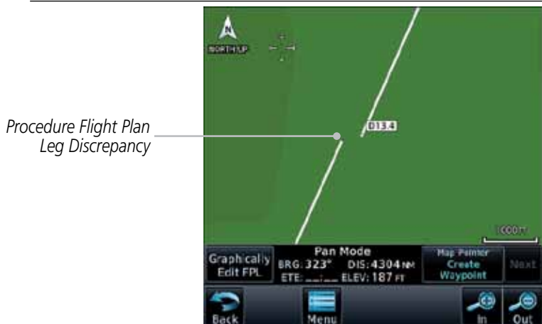
Figure 4-15 Procedure Flight Plan Leg Position Difference
