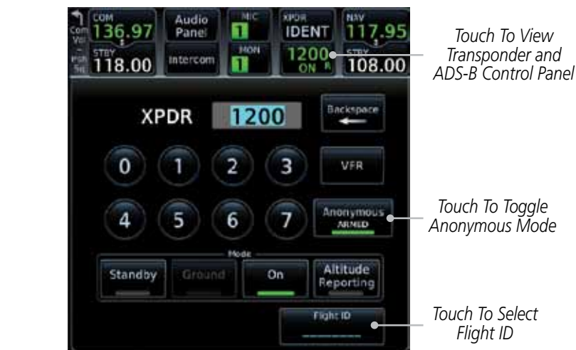
Figure 2-11 ADS-B/Transponder Control Panel
